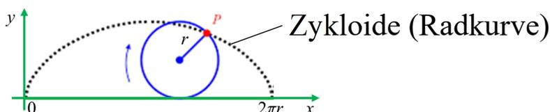
$$\begin{aligned}(x'(t))^2 + (y'(t))^2 &= r^2(1 - \cos t)^2 + r^2 \sin^2 t = r^2(1 - 2 \cos t + \cos^2 t + \sin^2 t) \\ &= 2r^2(1 - \cos t) \neq 0 \text{ in } (0, 2\pi),\end{aligned}$$
