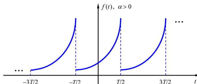
$$\Rightarrow T(t) = \sum_{k=-\infty}^{\infty} c_k e^{jk\omega t} = \begin{cases} f(t) & \text{für } t \neq \frac{T}{2} + kT \\ \frac{1}{2}(e^{\alpha T/2} + e^{-\alpha T/2}) & \text{für } t = \frac{T}{2} + kT \end{cases}$$
