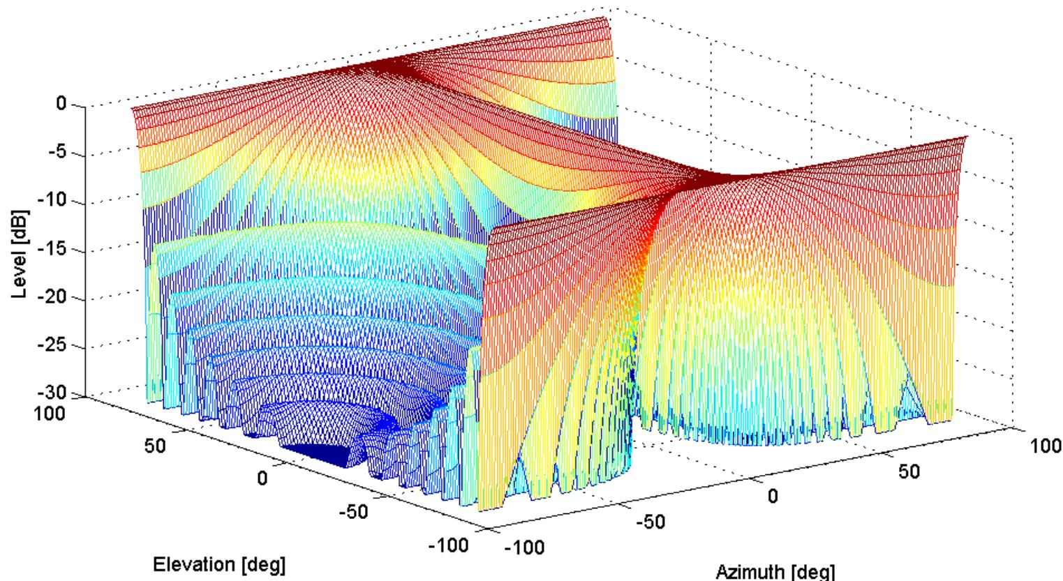
Typical beam pattern  $\tilde{B}(\varphi, \theta)$  of a linear aperture
