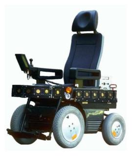
Fig. 3. The autonomous wheelchair Rolland that was model-checked for mode confusion problems. Photo: Rolf Müller
